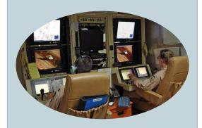
Automatic UAV flies on pre-determined routes, and the remote pilot intervenes in case of unforeseen events not programmed in pre-determined operation.
